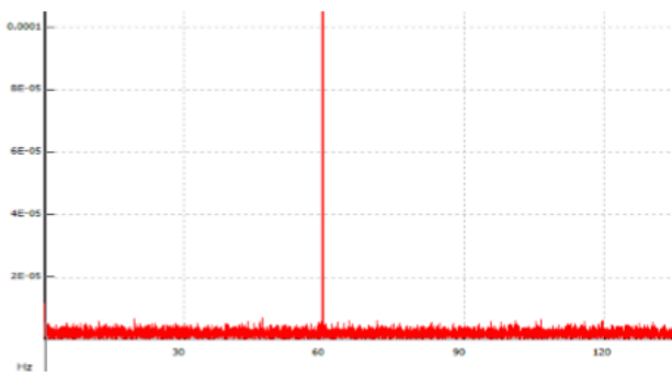
Figure 1. FFT Frequency analysis of EMF data. 60Hz peak frequency.
